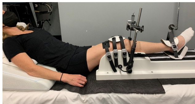
Figure 1. Patient set-up in GNRB device
